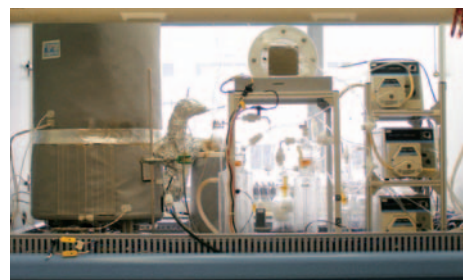
HHLT (thermo-chemical and electrolytic Hybrid Hydrogen process in Lower Temperature range) 工学試験実験装置
